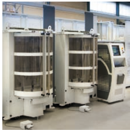
Ergonomical loading station ensures easy access to the pallet centre
