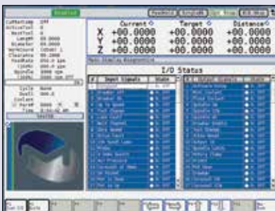
Diagnostic Display I/O Status
