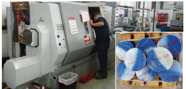
A pallet of raw steel, right, before machined on the Haas SL-30 featuring embedded chip trays and high-volume coolant systems for efficient chip removal.
