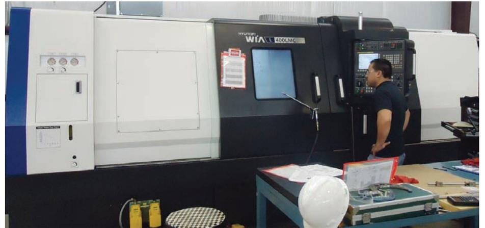
The Hyundai WIA L400-LMC CNC lathe with a FANUC-i control and a driven tool speed of 4,000 RPM.
