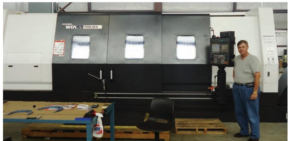
Jim McKee, President, Triple J Coil and Tubing Products with the Hyundai WIA L700 LMA with a maximum spindle speed of 1,500 RPM and box guideways.
