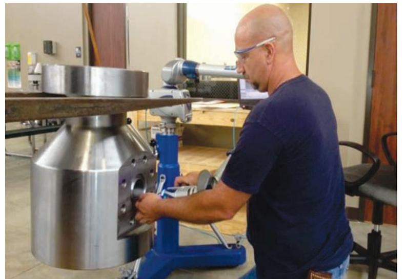
The FARO Edge portable CMM performing a 3D inspection.
