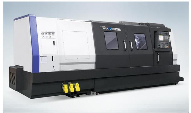
The L400LMC lathe with C axis and driven tools is one of three HyundaiWia turning machines used by Cosmopolitan Engineering
