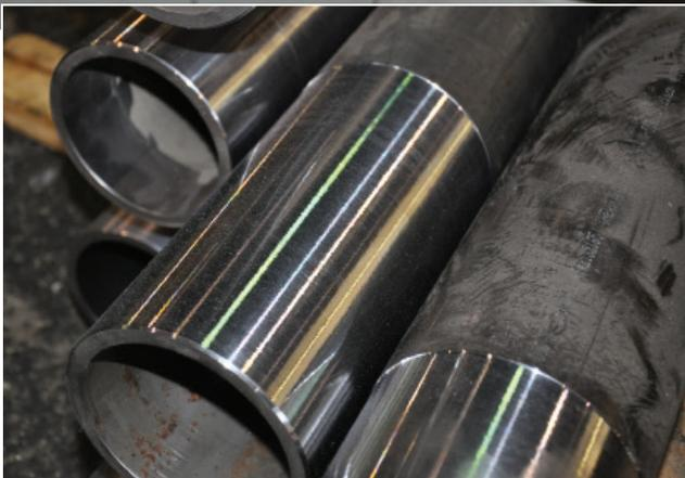
Although this is a rather basic contouring head application on a boring mill, it shows how programmable heads alter the effective cutting edge diameter to create a chamfer, "turn" an OD and generate a radius. This tube is part of a large L-shaped welded assembly that couldn't be turned on a lathe.
