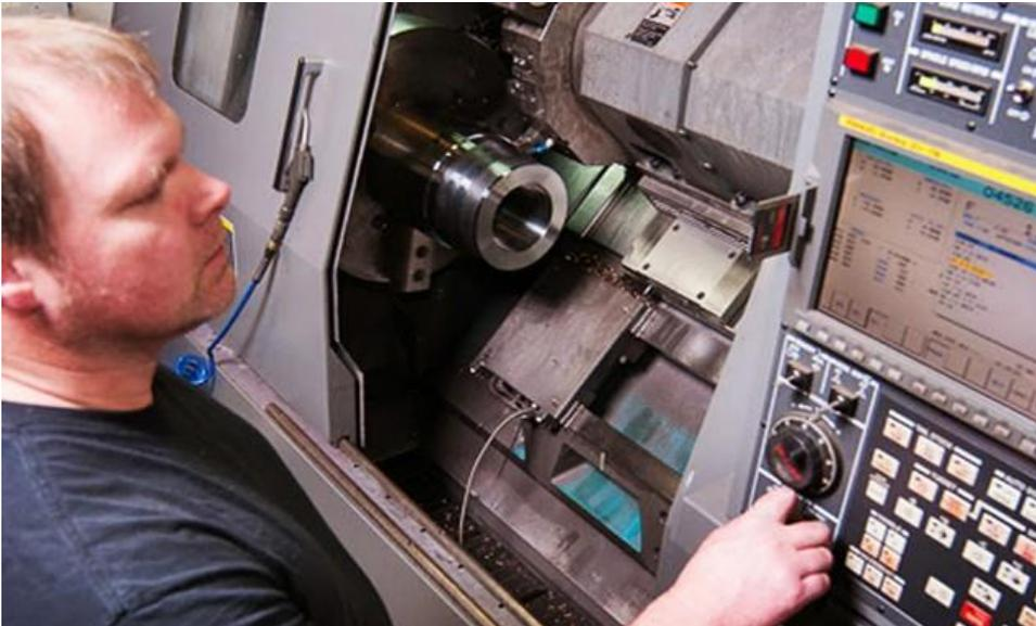
An operator at Seeley Machine programs a Hyundai WIA SKT Turning Center for a large diameter part
